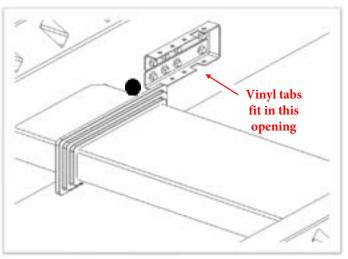
• Slide your vinyl trim rings over your 2x8 profile as pictured. Ensure the "tabs" on the inside of the vinyl trim rings line up with the holes on the metal bracket openings.
